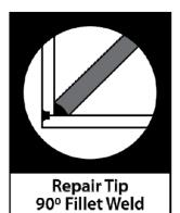
Repair tips are used for crack repairs, filling small holes, spot welding, for reaching tight areas, and for prototyping. Because of their conical shape, the repair tip and prototyping tip offer similar types of welds. Choose the size that best suits your application.
