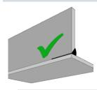
Welding rod should penetrate to the root side of the parent plastic Since molten welding rod did not penetrate the root, a poor weld will result
